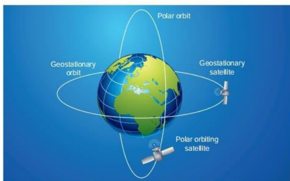
Figure 6.21 Polar orbit and geostationary satellite
